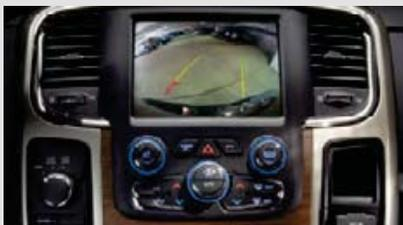
The new, large available 8.4-inch touch-screen radio in select new 2013 Ram Heavy Duty models now offers full-color displays, including three-dimensional imaging of landmarks and city modeling. New Active Grid Lines in the display are another Ram advantage — they're invaluable when backing up, changing with each steering wheel movement. Now you can easily and accurately align your hitch to the trailer, with no need to hop out to double-check, or bother with a spotter.
