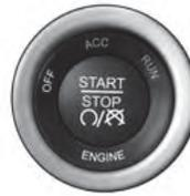
This feature allows the driver to operate the ignition switch with the push of a button, as long as the Remote Start/Keyless Enter-N-Go™ Key Fob is in the passenger compartment.
