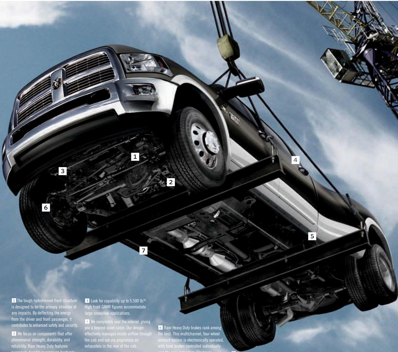
**1** The tough hydroformed front structure is designed to be the primary absorber of any impacts. By deflecting the energy from the driver and front passenger, it contributes to enhanced safety and security.
