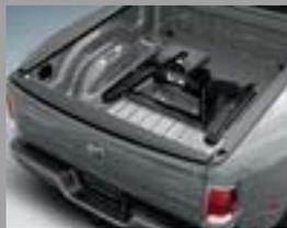
Available Mopar Fifth-Wheel Hitch enables super-tough trailer towing with authority. Options include a hitch with sliding rails or one that mounts directly into the optional Fifth-Wheel/Gooseneck Prep Package mounts, saving time and effort.
