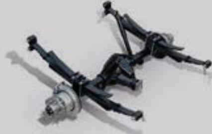
**3500: THE STANDARD HOTCHKISS LEAF SPRING REAR SUSPENSION** capably meets every need for payload and occupant comfort. For Ram 3500 Dually models, the spring package employs separate auxiliary leaves—engineering that helps enhance the rear handling and which also allows for higher payloads.
