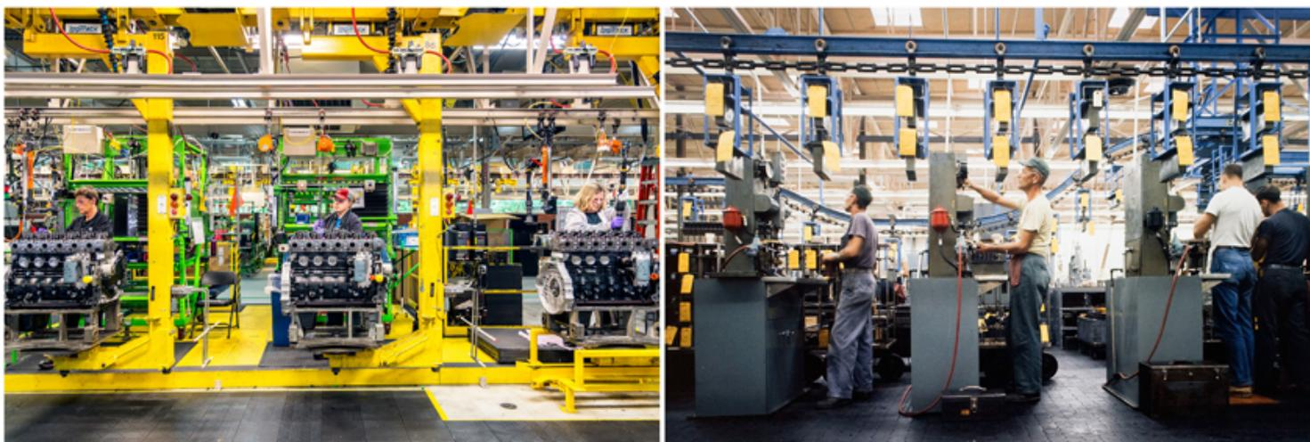
Assembling engines for Dodge Ram trucks at a Cummins plant today; workers on one of the company's original assembly lines in
