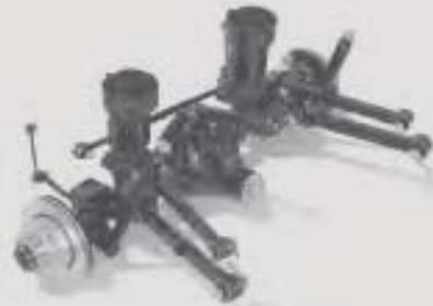
THE NEW AVAILABLE AUTO-LEVEL REAR AIR SUSPENSION SYSTEM\* FOR RAM 2500 is based on the available Active-Level™ Four-Corner Air Suspension System introduced by Ram 1500, here in an operator-selectable two-mode configuration to accommodate the higher GCWRs of the weight class.
