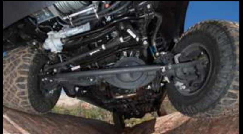
**ELECTRONICALLY DISCONNECTING FRONT SWAY BAR | POWDER-COATED STEEL BUMPERS | FUNCTIONAL TOW/RECOVERY HOOKS | HEAVY-DUTY STEEL UNDERCARRIAGE PROTECTION | BILSTEIN MONOTUBE SHOCKS**
