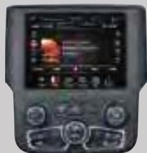
**UCONNECT 8.4A.** With 8.4-inch full-color touch-screen display; AM/FM with remote USB/SD; iPod integration; Bluetooth connectivity for hands-free phone;<sup>[10]</sup> Streaming Audio, Voice Command,<sup>[11]</sup> Voice Text Reply;<sup>[6]</sup> also includes dealer-activated navigation; HVAC control integration; smartphone connectivity; rearview camera<sup>[7]</sup>-ready; SiriusXM Satellite Radio<sup>[9]</sup> Available: remote CD player.
