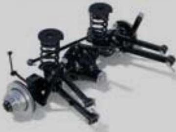
**2500: THE CLASS-EXCLUSIVE<sup>(1)</sup> FIVE-LINK COIL SPRING REAR SUSPENSION**, standard on Ram 2500, is revolutionary in the heavy-duty pickup segment. Engineered to spec, it provides outstanding ride/handling characteristics and beyond-dependable hauling and payload capability, irrespective of load.
