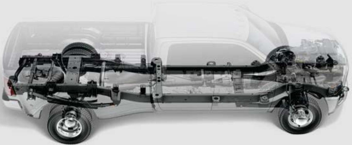
Ram Heavy Duty model frames employ an integrated rear axle crossmember with provisions for an available fifth-wheel and gooseneck hitch. Mounting provisions are integrated into the production box floor and include fifth-wheel pucks, gooseneck bolt plates and gooseneck center castings, with the 7-pin wiring connector mounted directly into the bed.
