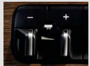
All-new for 2013: the Integrated Switch Bank. Conveniently mounted in the dashboard, it offers fingertip management of the standard ESC<sup>(4)</sup> system, the available Trailer Brake Controller (if equipped), and the Tow/Haul Mode, with controls for other available features — such as heated/ventilated seats, heated steering wheel, etc.
