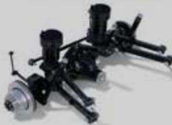
**3500: THE AVAILABLE AUTO-LEVEL REAR AIR SUSPENSION SYSTEM** is engineered to meet the ultra-heavy-duty assignments typically met by Ram 3500 single-rear-wheel and dual-rear-wheel models. In this version, leaf springs are augmented with the air springs mounted on top of the axle. The result: air springs work with the leaf springs for ideal handling and performance while hauling big payloads.
